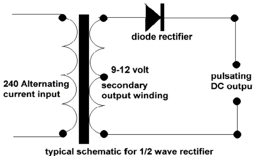
Others with a little imagination can see it as a half wave dc power rectification schematic .
